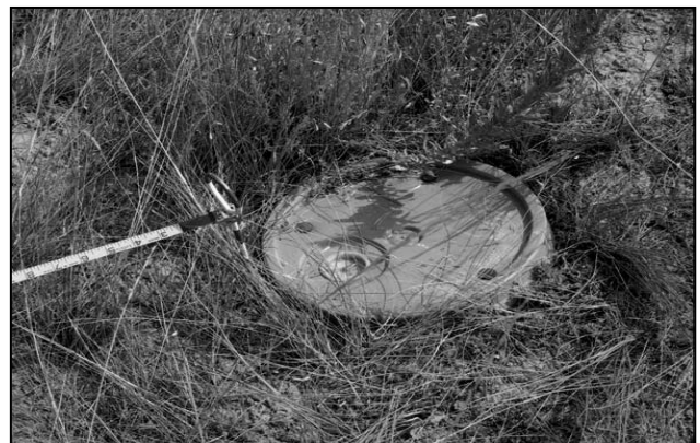
Photo 22: Five-gallon bucket lid used to mark the beginning point of a transect. The tape measure stretched out from this point can also be seen.
